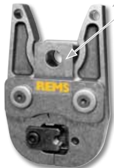
Cropping tongs with reversible cutting inserts for steel, stainless steel, M 6–M 12, up to strength class 4.8 (400 N/mm 2 ).
