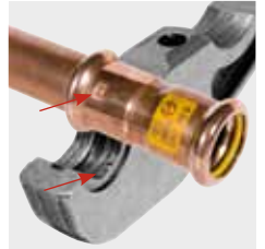
Example REMS pressing tongs M: Impression "M" on pressed fitting for traceability according to EN 1775:2007
